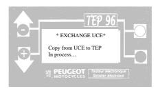
4. Following this screen the TEP 96 displays "Do you want to copy parameters? NO/YES" press NO to save the ECU parameters and return to the main menu
